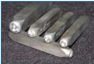
For light to medium indenting jobs, Triumph type can indent up to 3/16" high characters on tin, aluminum and other soft metals. The spring mortise lever on the hand-style type holder secures and provides quick type changes. Select among three holder sizes. A nick on the body of the type permits easy orientation of characters in the Triumph holder. The type can also be used with Shank Type holders in impact presses or with Dove Tail holders in roll marking machines.
